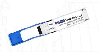
The central wavelengths of the 4 CWDM channels are 1271, 1291, 1311 and 1331 nm as members of the CWDM wavelength grid defined in ITU-T G.694.2. It contains a duplex LC connector for the optical interface and a 38-pin connector for the electrical interface. To minimize the optical dispersion in the long-haul system, single-mode fiber (SMF) has to be applied in this module.
