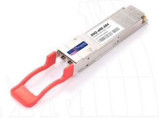
The central wavelengths of the 4 CWDM channels are 1271, 1291, 1311 and 1331 nm as members of the CWDM wavelength grid defined in ITU-T G.694.2. It contains a duplex LC connector for the optical interface and a 38-pin connector for the electrical interface. To minimize the optical dispersion in the long-haul system, single-mode fiber (SMF) has to be applied in this module.
